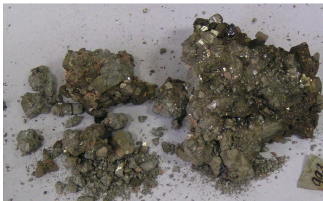
Fig. 1. Altered Pyrite due to ferro-sulphides composition in the hygroscopic environment
