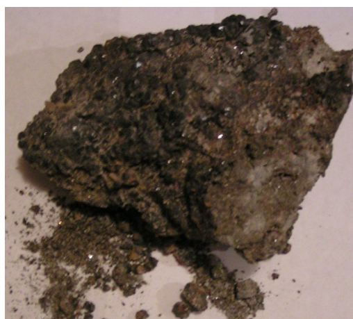
Fig. 6. Altered sphalerite due to pyrite and marcasite paragenesis
