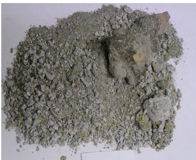
Fig. 7. Physically and chemically altered chalcopryite
