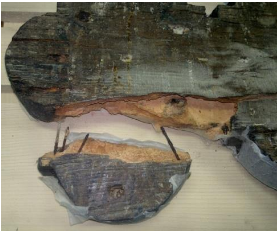
2. Cross – consolidation with iron nails; detail
