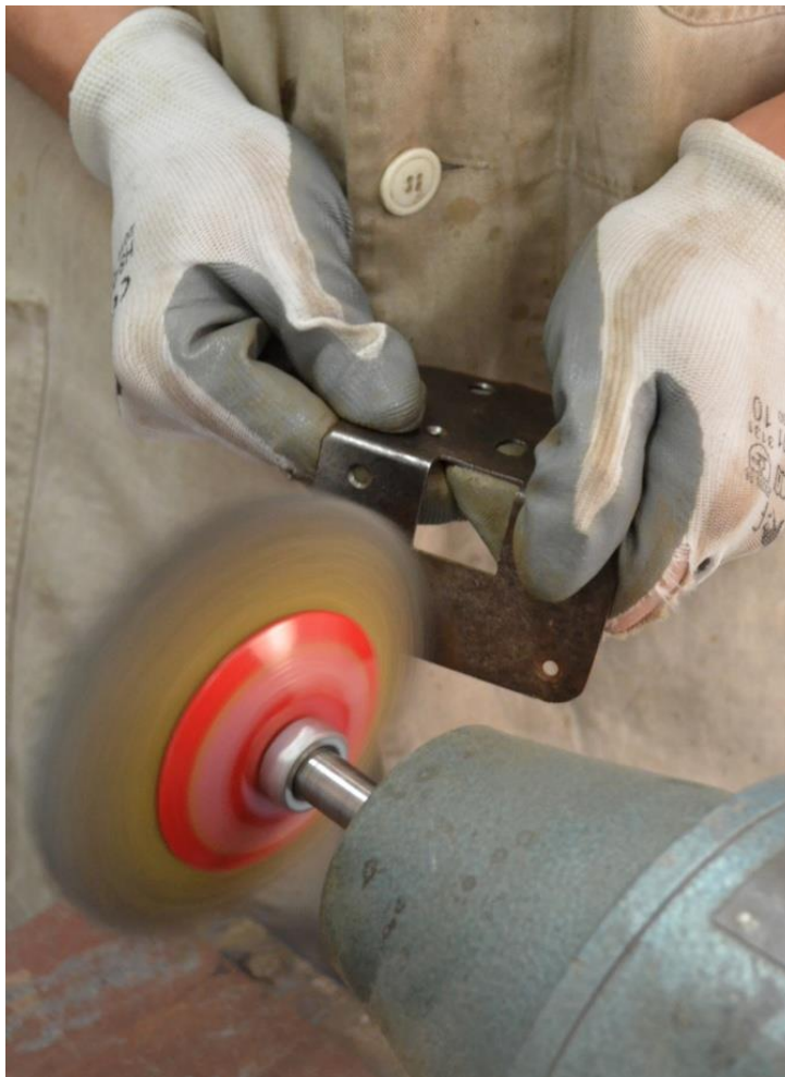
11. Detail; mechanical cleaning of the metallic elements
