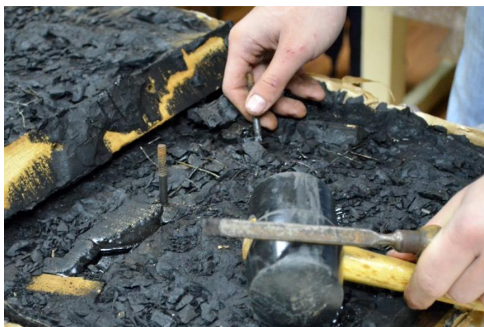
6. Detail; the removal of the metallic elements
