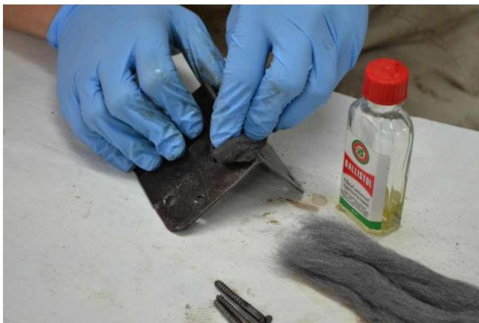
12. Detail; passive process of the metallic elements
