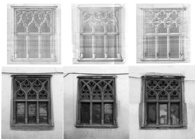
Fig. 11. Cluj, former Dominican convent, design patterns of the refectory windows as drawn for the 1902 restoration project and solution achieved
