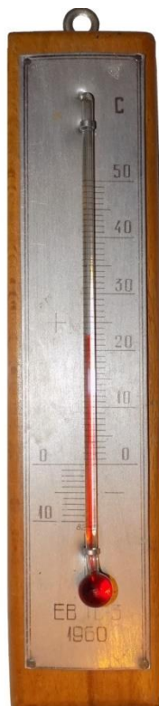
Photo 5. Alcohol thermometer, used in the past at the Brukenthal National Museum to determine the temperature values in storage and exhibition spaces - 1960
