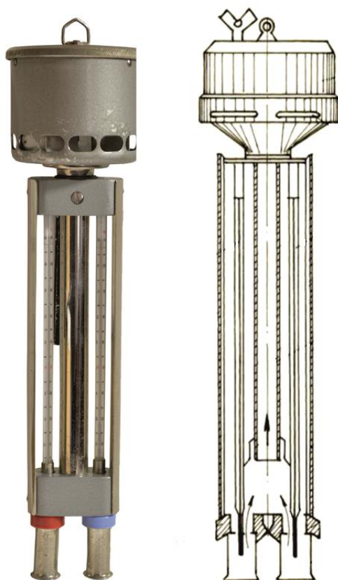
Fig. 1. The “Asman” type psychrometer – (sketch after the Bancea, 2009)
