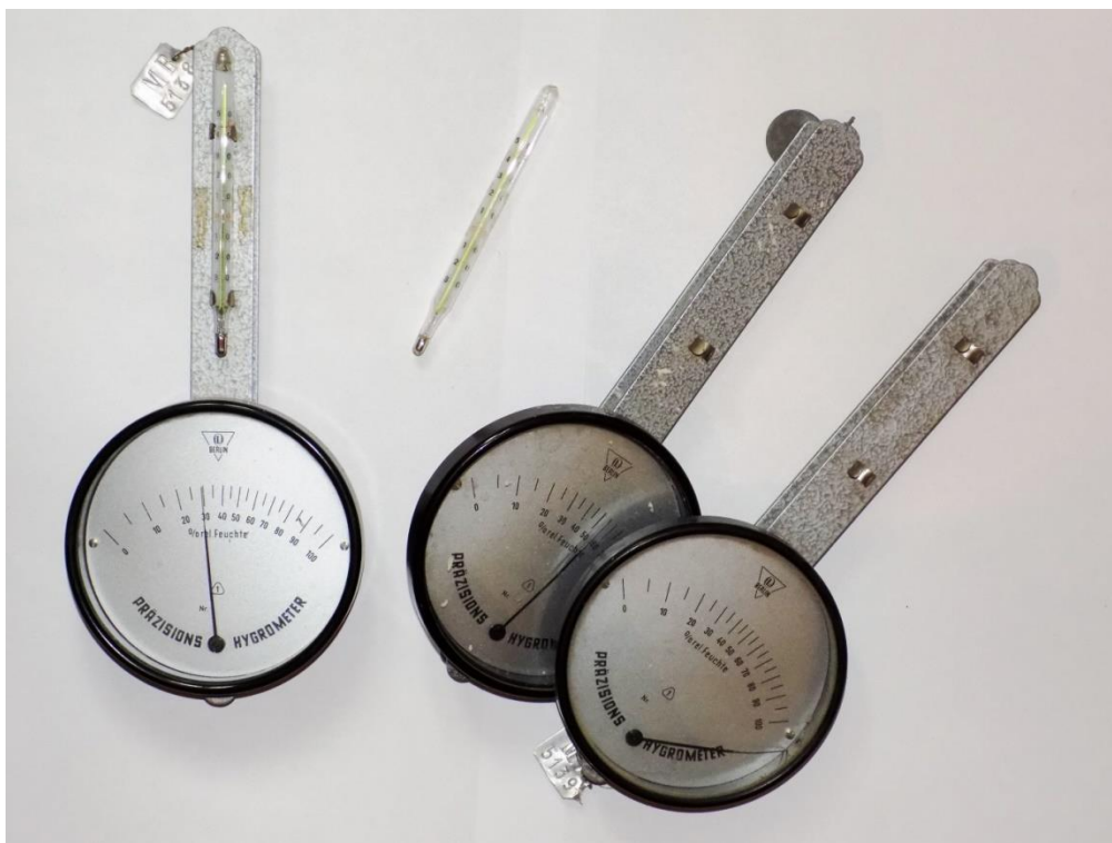
Photo 4. "Prazisions" hygrometers - equipped with a common mercury thermometer, becomes a thermohygrometer
