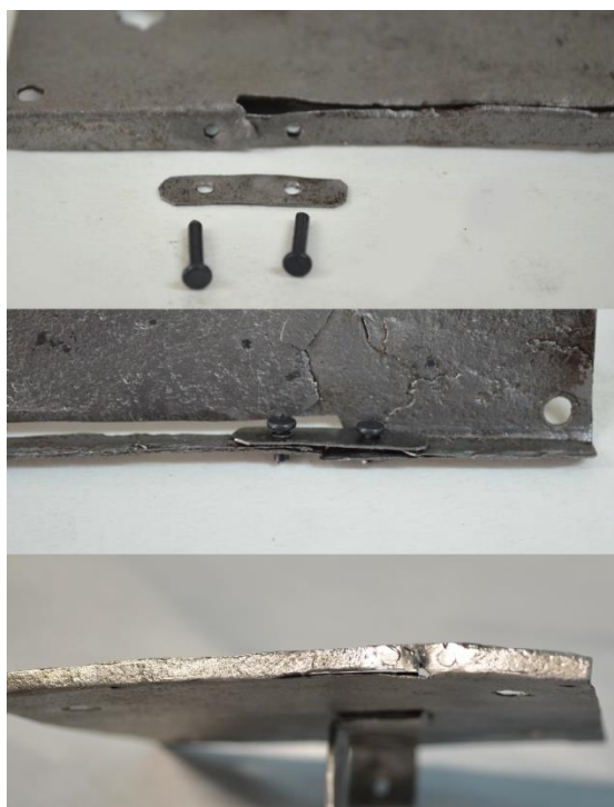
5. Detail of the method used to attach the fractured plate
