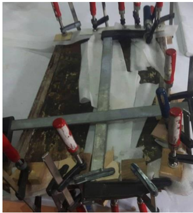
11 Gluing of upper and lower wands
