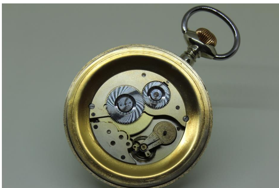
19. movement view after cleaning, without crystal
