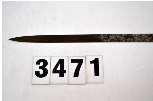
3. Detail of the blade corosion products
