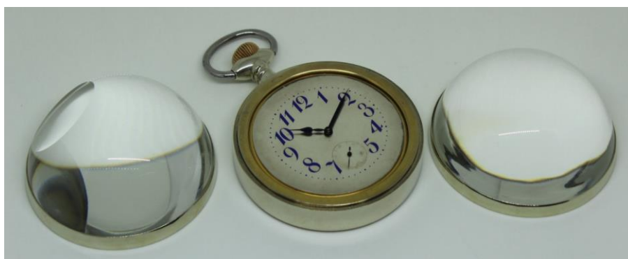
18. movement and dial mounted into case, without crystals
