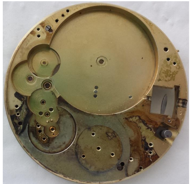
4. movement plate view, before restoration
