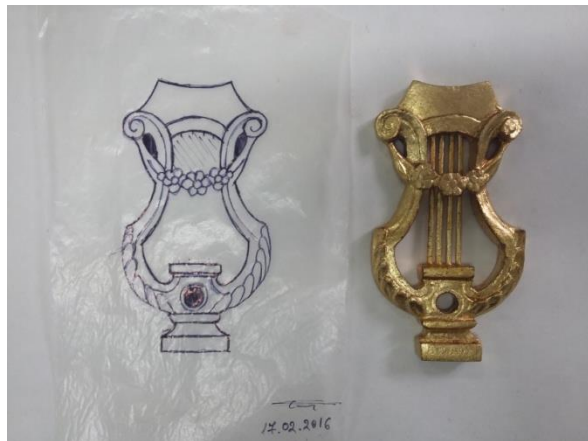
13. Detail, the new lyre-shaped support made for holding the clock's case, gilded and modeled after a clock of the same type
