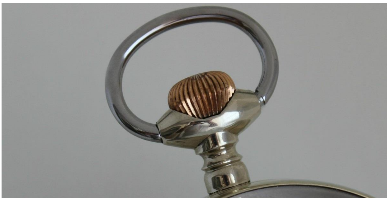
7. new lathe made pendant ring
